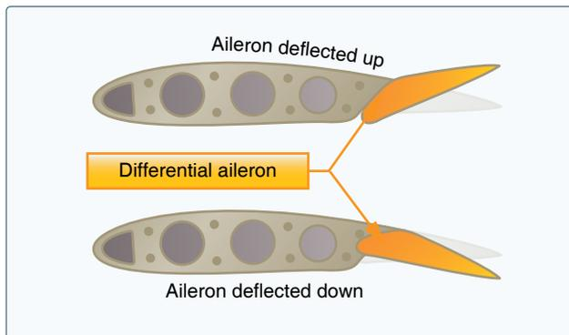
Figure 6-6. Differential ailerons.
