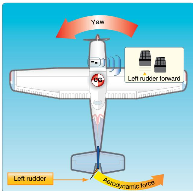
Figure 6-15. The effect of left rudder pressure.
