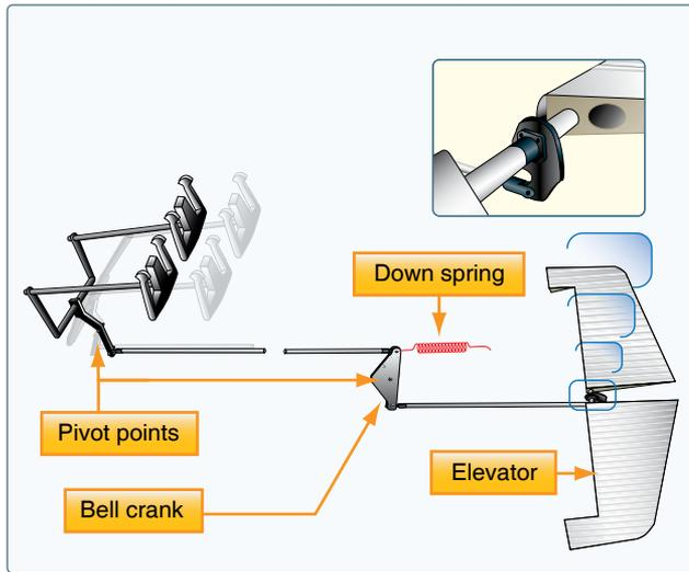
**Figure 6-12.** When the aerodynamic efficiency of the horizontal tail surface is inadequate due to an aft CG condition, an elevator down spring may be used to supply a mechanical load to lower the nose.
